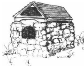
Oven with brick dome covered with fieldstones Kamouraska Blanchette Collection, CCFCS Ar- chives, no. 194
