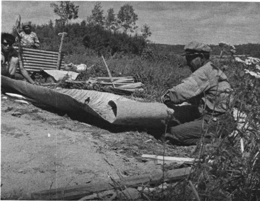
Plate 8 Unrolling the bark beside the building bed
