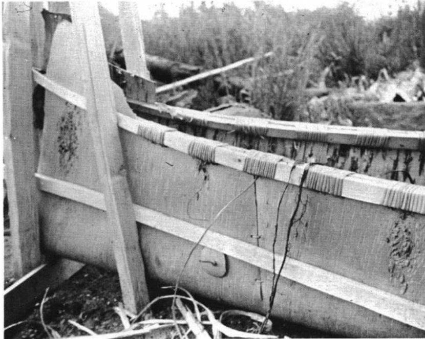
Plate 23 Lashings: note the restraining disc used to sheer the gunwales
