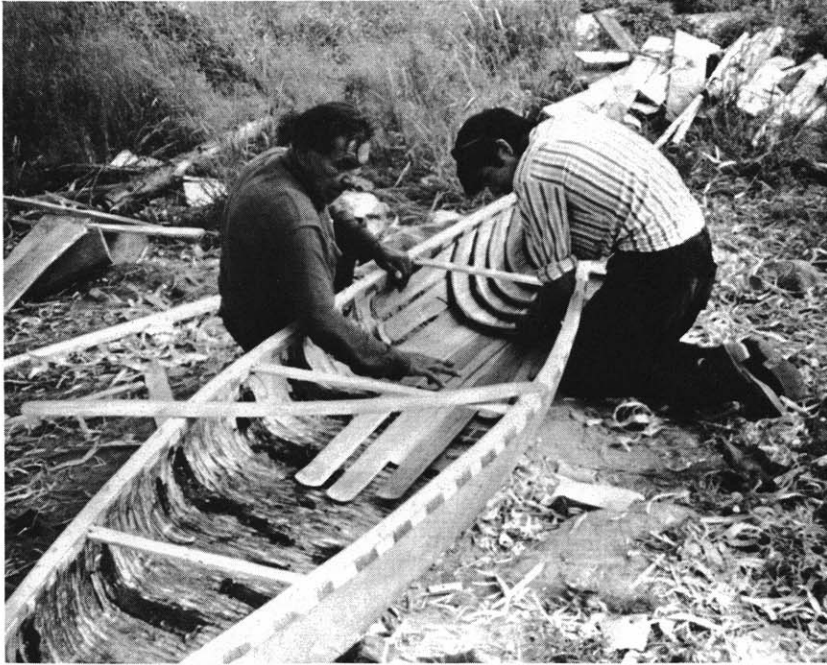
Plate 31 Installing the sheathing and the ribs
