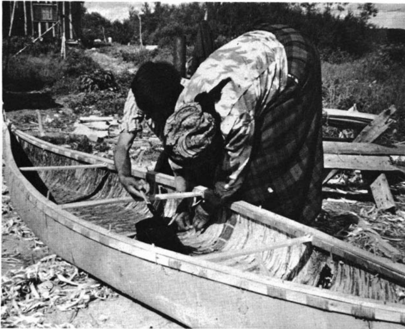
Plate 29 Caulking the inside of the canoe
