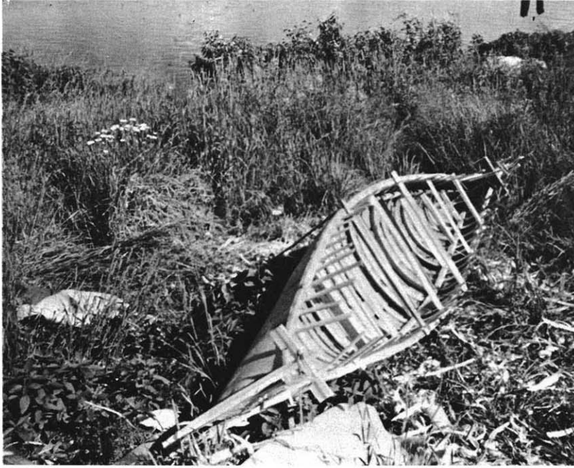
Plate 27 The ribs drying in their canoe "mould"
