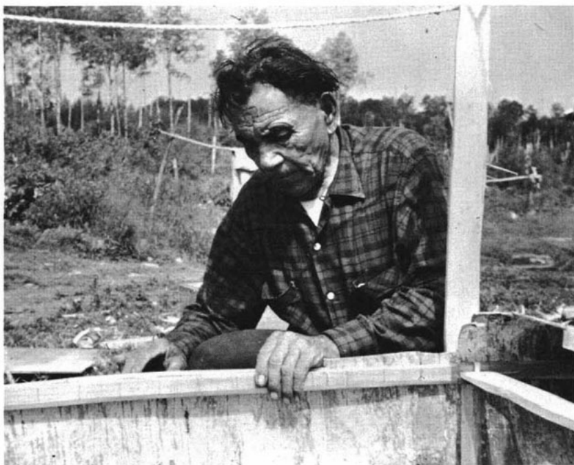
Plate 21 Trimming away the surplus bark
