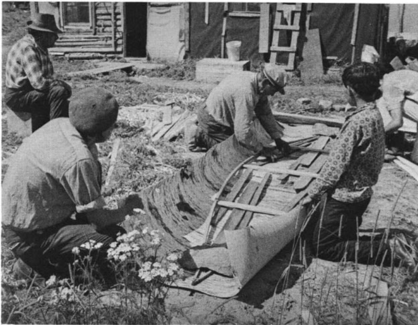
Plate 10 Adding split planking to protect the bark
