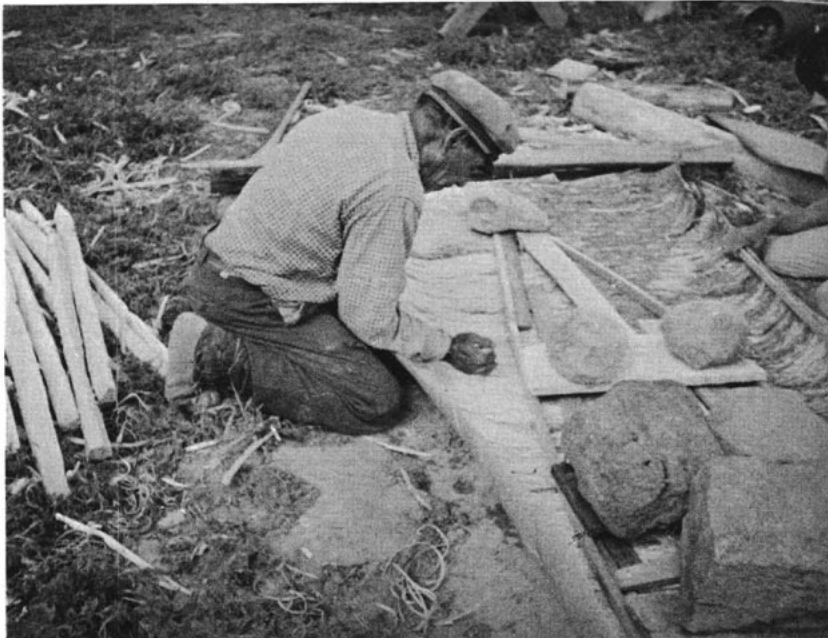
Plate 12 Slitting the bark from edge to frame
