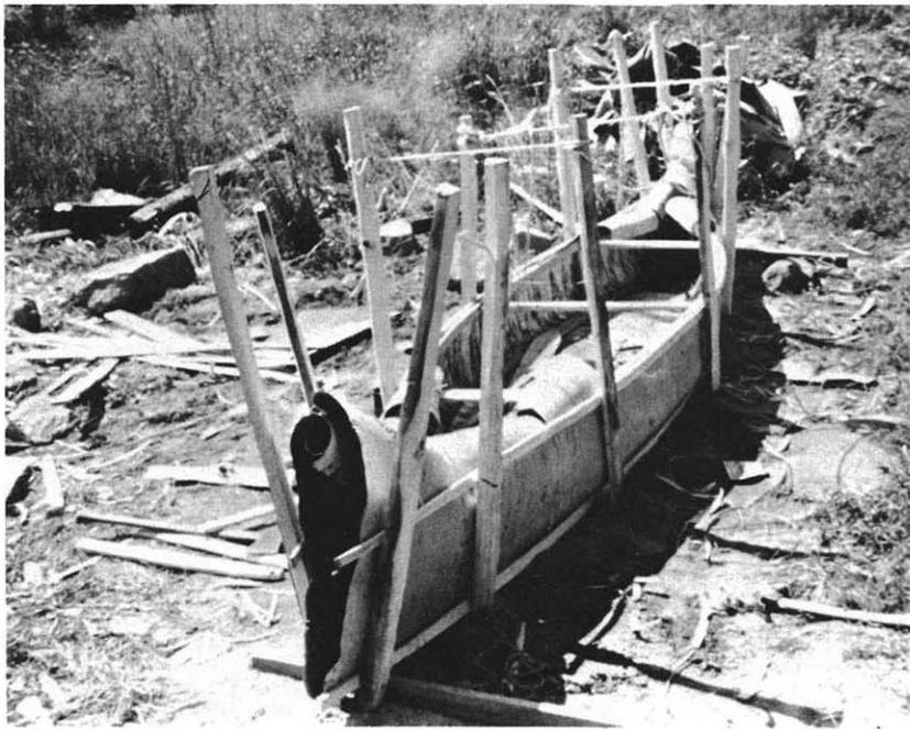
Plate 20 The building frame raised to gunwale height
