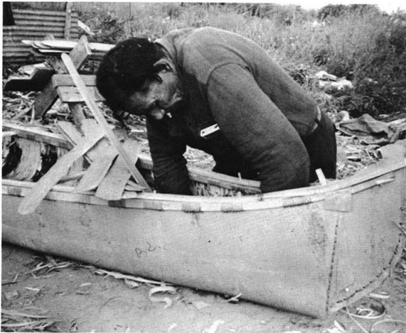
Plate 30 Lashings of the extension and bark reinforcing gusset
