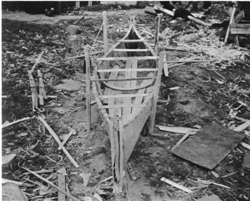
Plate 26 Bracing the canoe with temporary thwarts, and inserting the first rib
