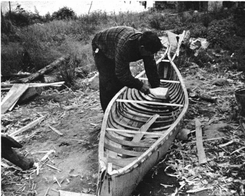
Plate 32 Tapping the ribs into place with a mallet
