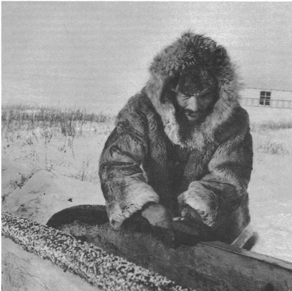
Plate 10. In order to facilitate sledge travel mudding was applied to the runners to form a base for icing which drastically reduced friction against the granular snows of winter.
